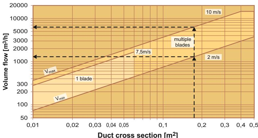
Diagram 1: Choosing of V<sub>max</sub> and V<sub>min</sub> via the duct cross section
